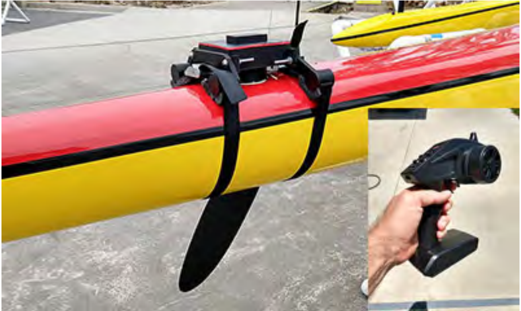
Fig. 2. A close-up of version three of the CoOP system mounted to the rudder assembly and the transmitter used to control the rudder (right corner).
